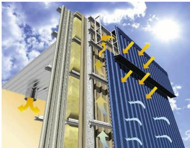
Figure 1.3 : Illustration du SolarWall (source: [www.solarwall.com](http://www.solarwall.com))
