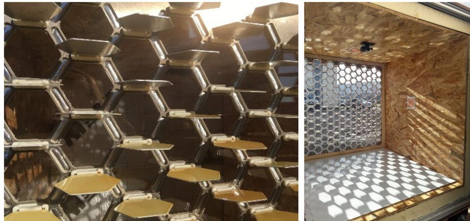
**Figure 11.** Photos of the Stegos 'glazing' configuration on the test box with claps positioned as solar caps and opened to a  $90^\circ$  angle. Camera fixed on the roof wall of the test box.
